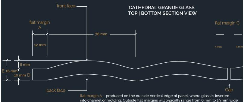
D - indicates thickness of flat section of glass
