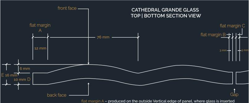
D - indicates thickness of flat section of glass
