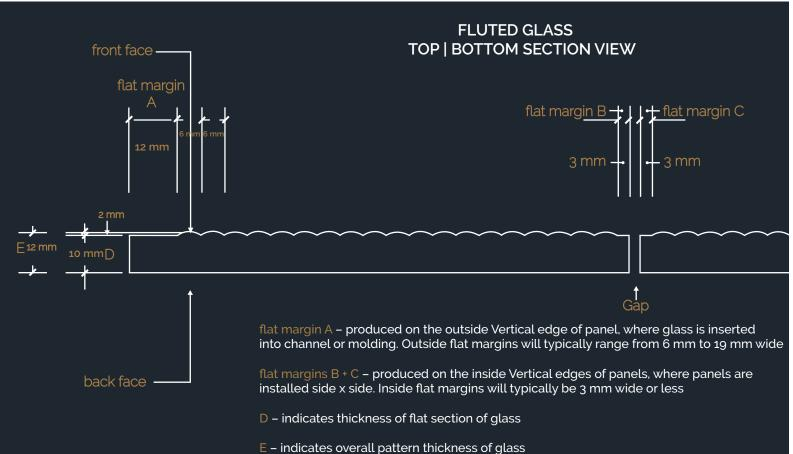
(Please note that the pattern thickness depth can vary slightly, from 1mm to 2mm, on some panels)
