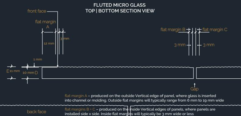
D – indicates thickness of flat section of glass
